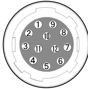
Figure 8-3 Pin Assignments for Power Input and Control I/O Receptacle
