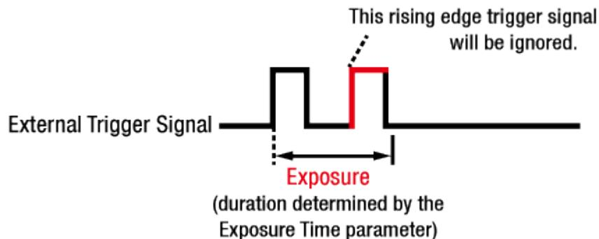
Figure 9-5 Trigger Overlapped with Timed Exposure Mode
