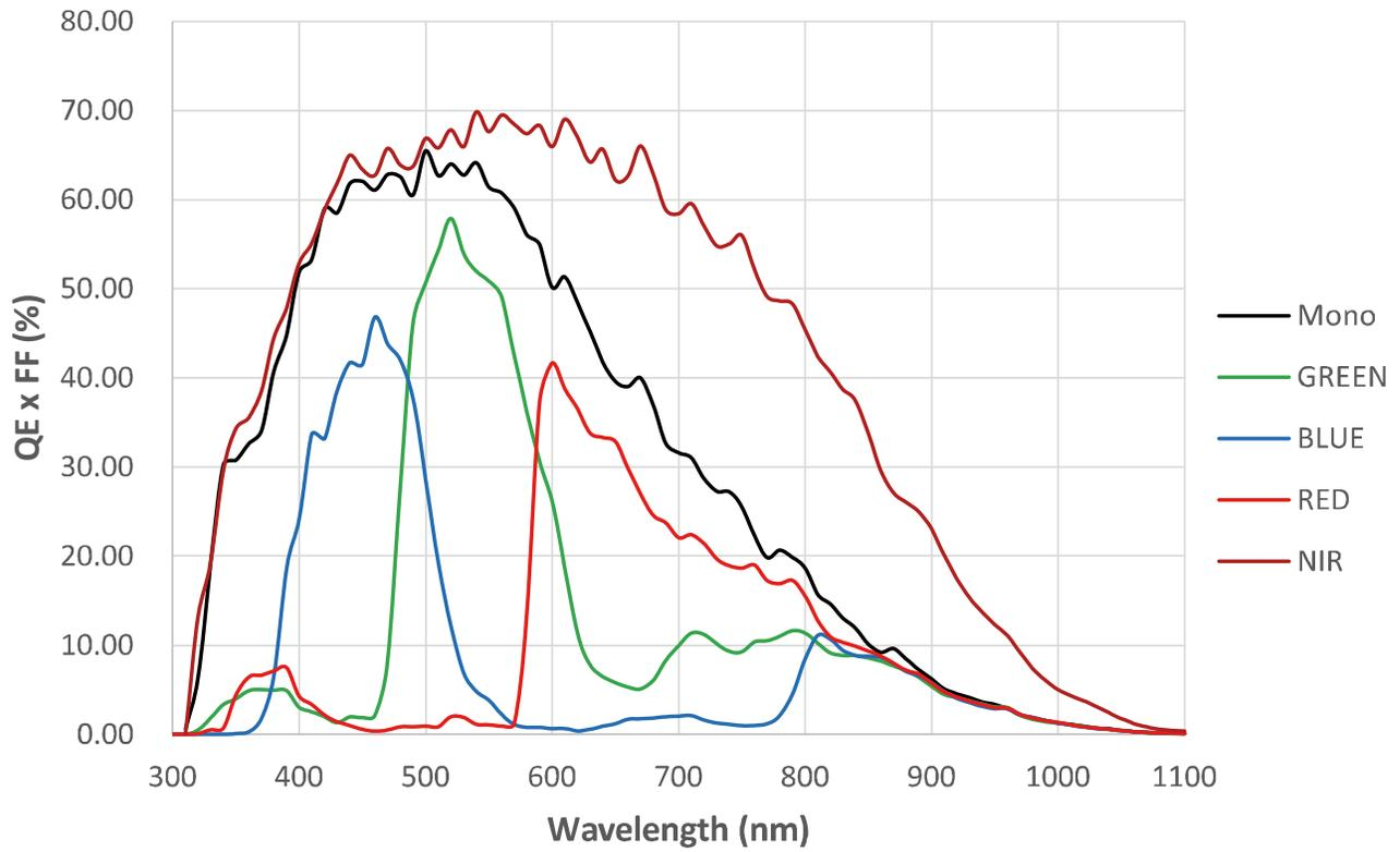
Figure 6-2 VC-25MX-M/C911 Spectral Response
