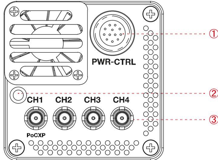
Figure 8-1 VC-25MX-91I with DIN 1.0/2.3-type Connectors
