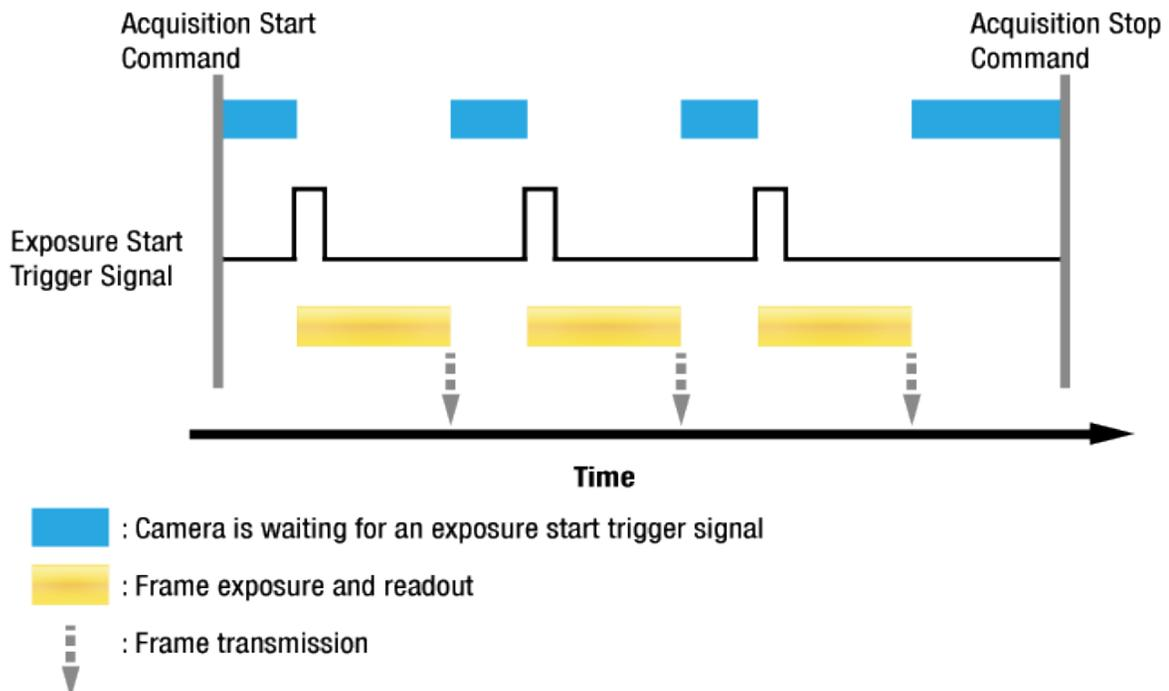
Figure 9-1 Exposure Start Triggering
