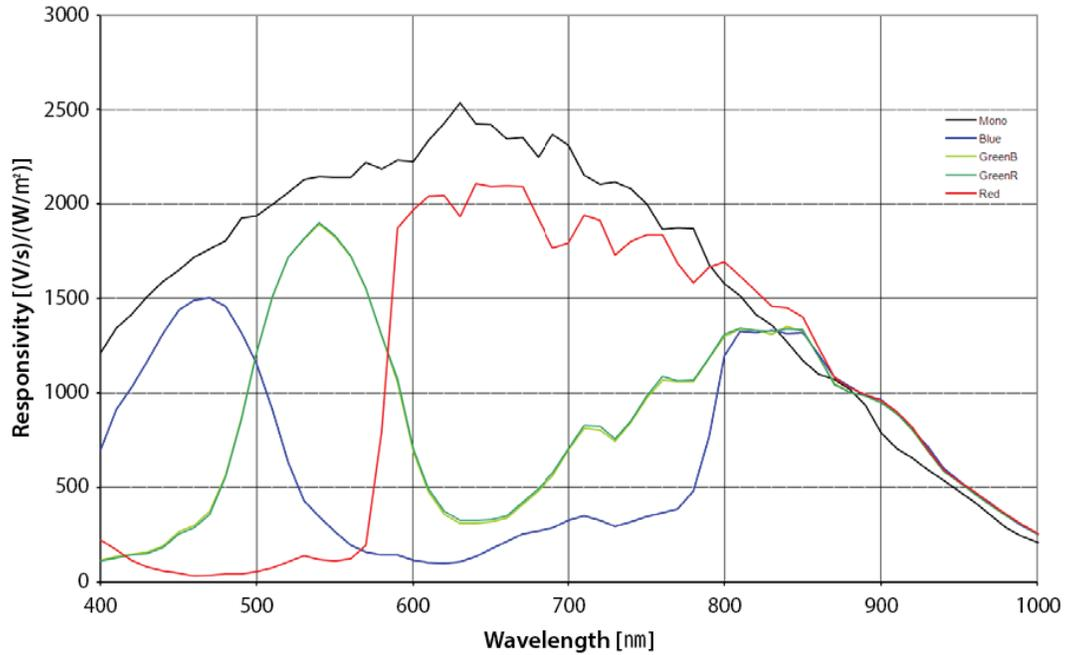
Figure 5.3 VC-25MX-72D 흑백 및 컬러 Spectral Response
