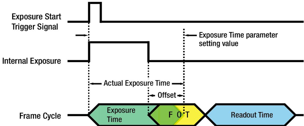
Figure 8.6 Real Exposure 를 적용한 Timed Exposure Mode
