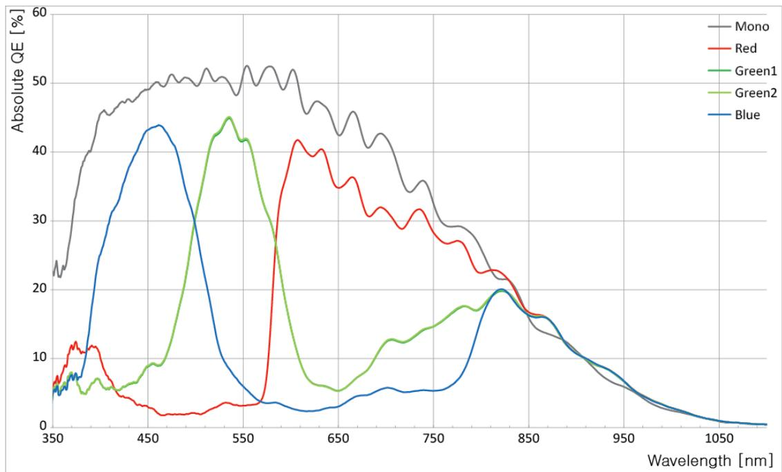
Figure 5.2 VC-12MX-180 흑백 및 컬러 Spectral Response
