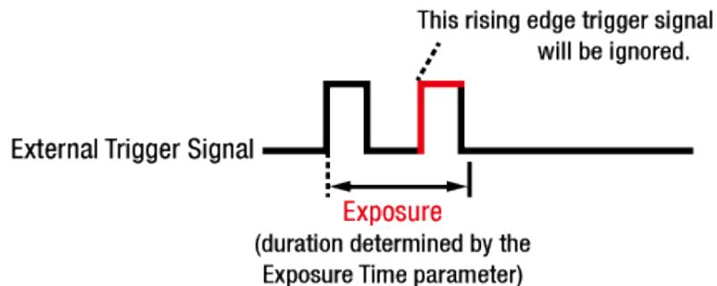
Figure 8.3 Trigger Overlapped with Timed Exposure Mode
