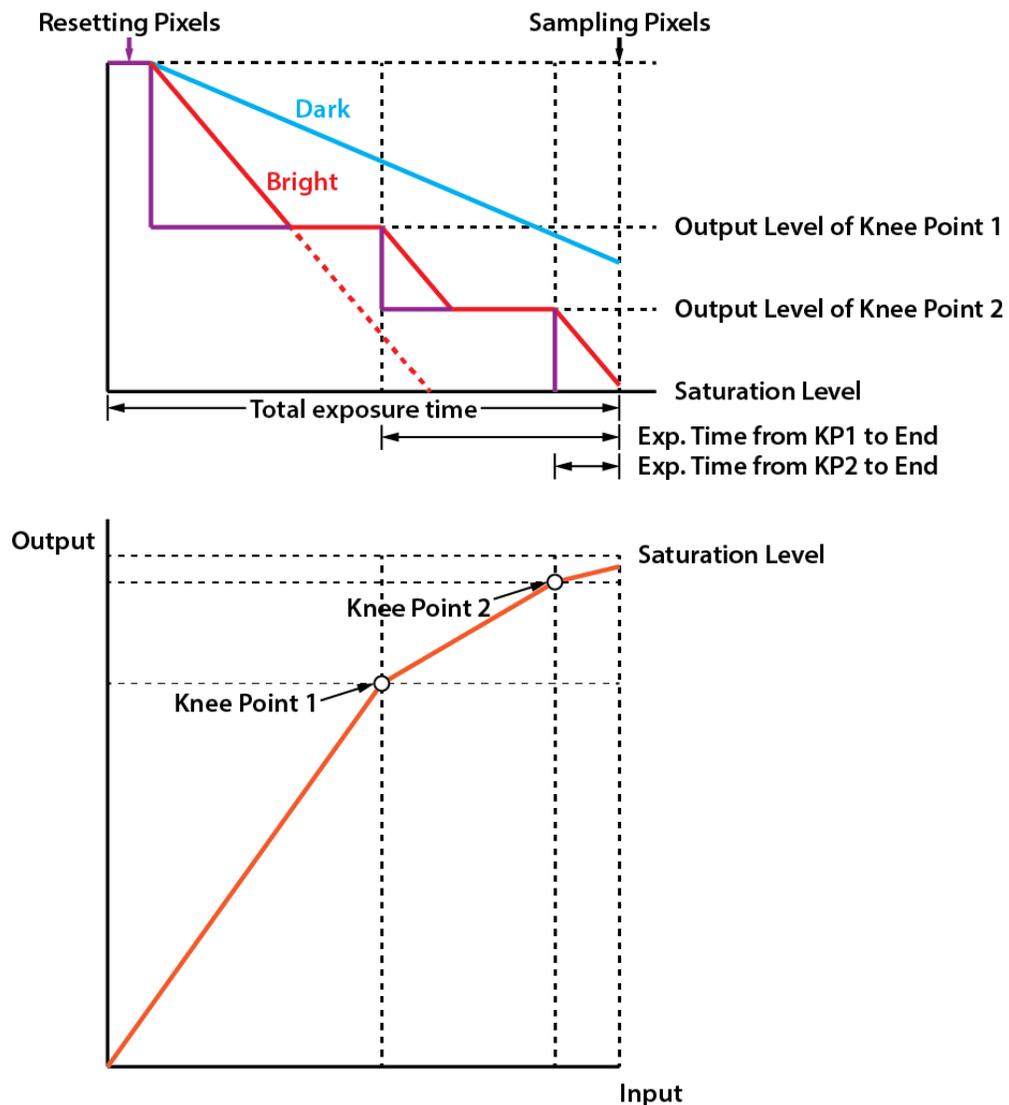
Figure 9.15 High Dynamic Range Concept Drawing
