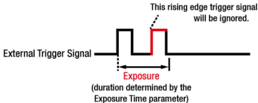
Figure 8.4 Trigger Overlapped with Timed Exposure Mode
