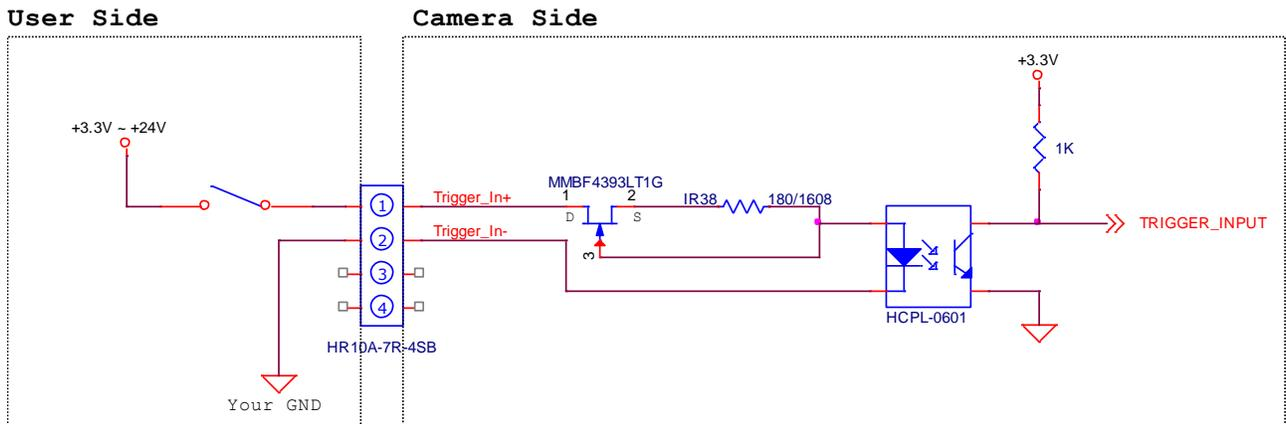
Figure 7.5 Trigger Input Schematic
