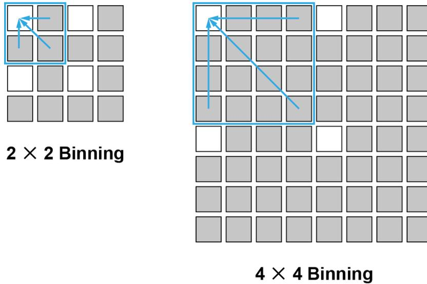
Figure 9.2 2 × 2 및 4 × 4 Binning
