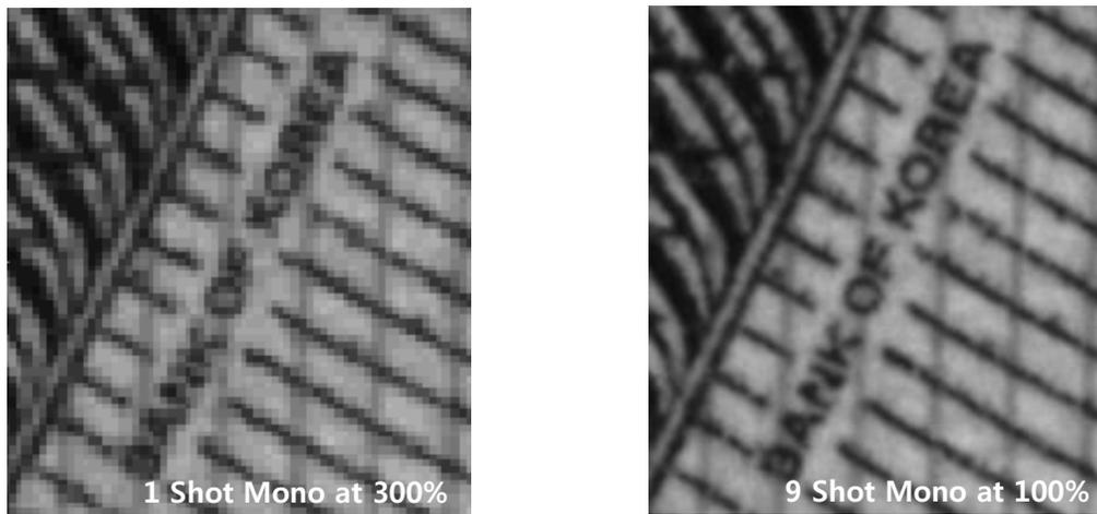
Figure 9.12 Standard (left) vs. 9 Shot Pixel Shifting (right)
