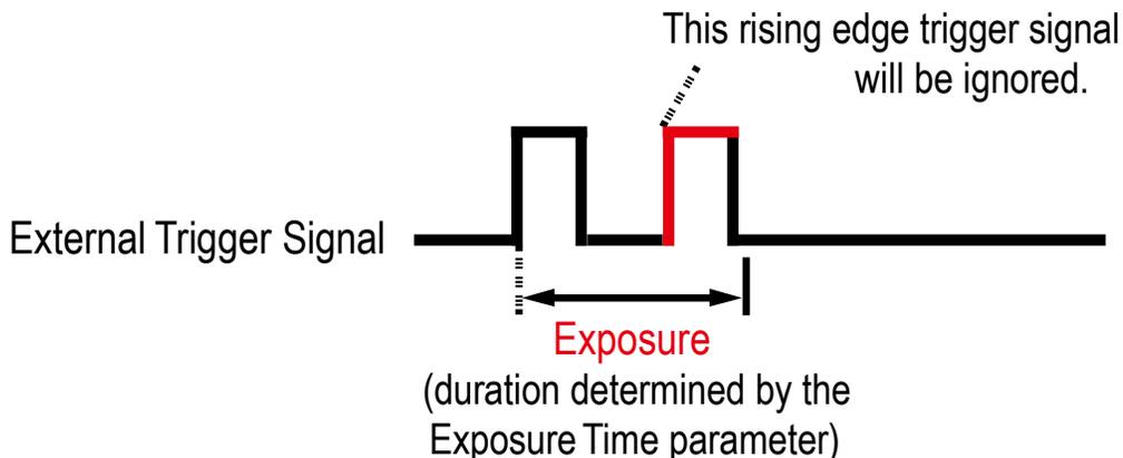
그림 8-5 Trigger Overlapped with Timed Exposure Mode
