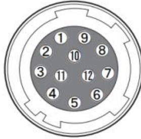
Figure 7.6 Pin Assignments for Power and Control I/O (VC-25MX2-150I-HS)
