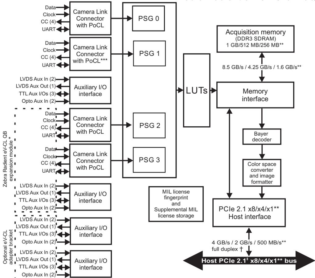
\* Note that, without the expansion module, this is a flow diagram of Zebra Radiant eV-CL SB or DB, depending on the number of camera link interfaces. With the expansion module, this is a flow diagram of Zebra Radiant eV-CL QB. eV-CL SB and DB are not upgradable to eV-CL QB; the eV-CL SB and DB do not have the required connector for the eV-CL QB module.
