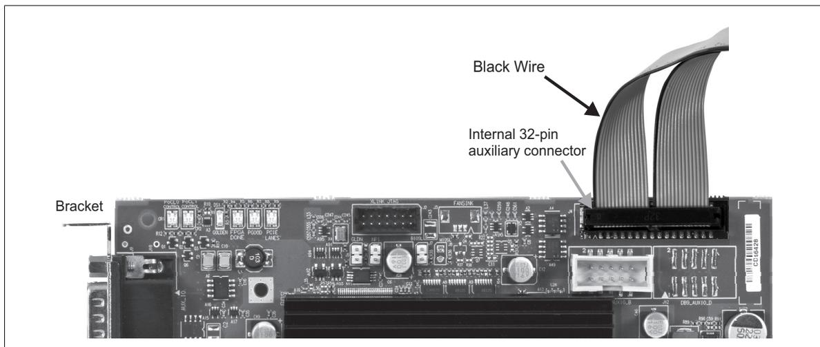
3. Slide the bracket of the cable adapter bracket into the opening at the back of the selected slot.
