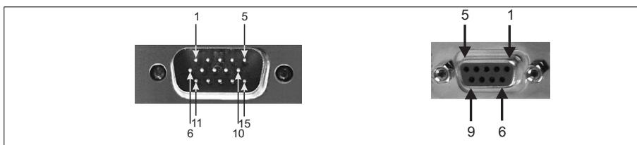
The dual HD-15 connector must be connected to the 32-pin internal connector and the DB-9 connector must be connected to the internal 10-pin connector<sup>†</sup>. On the cable adapter bracket, the connectors are panel mount connectors.
