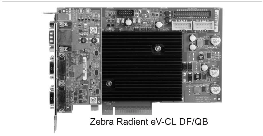
❖ Note that older versions of Zebra Radiant eV-CL included a fan. This has been replaced with a heat sink in newer versions.
