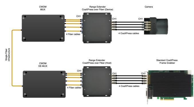
**NOTE:** Channel 1 (CH1) must have a duplex fiber connection (Or BIDI SFP with single fiber cable) while other channels can have a simplex fiber connection from device side to host.
